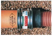
2 Place BAND-SEAL on the clay pipe and butt pipes together. Slide BAND-SEAL over bushes until edge of bush is level with edge of BAND-SEAL. No lubricant required.
