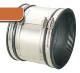
Naylor Extra Wide Couplings have a width of 300mm which allows a greater tolerance when cutting larger diameter pipes. The increased width also accommodates the greater movement of the joints associated with the depths at which these large diameter pipes are laid.
