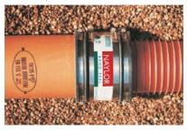
**3** Tighten clamp bands first, then the shear band. After BAND-SEAL assembly, carefully tamp bedding under and around pipes.
